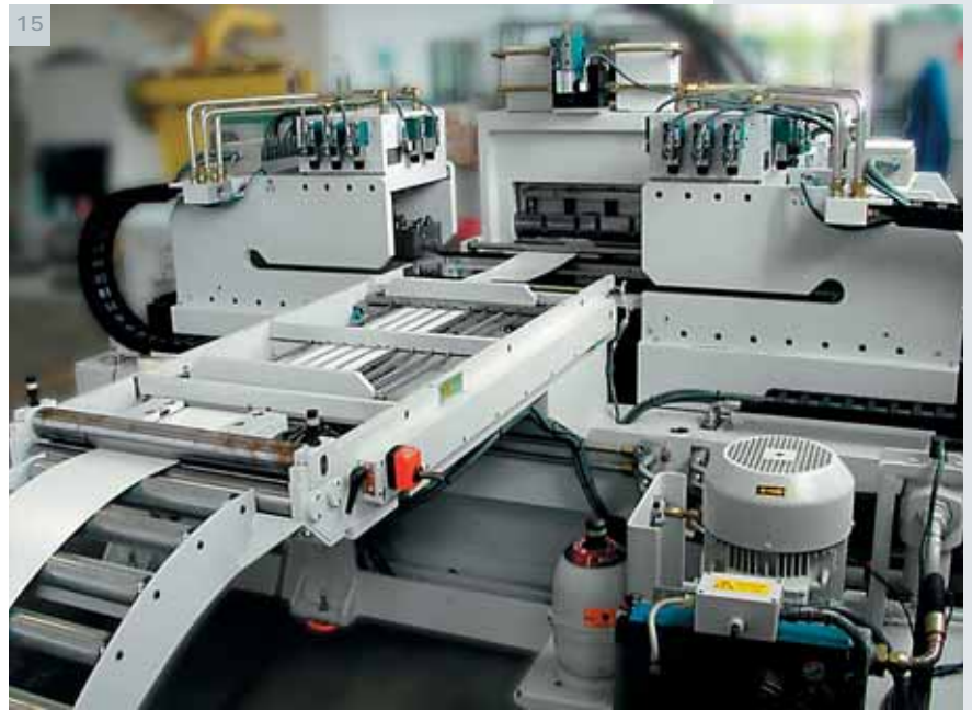
Picture 14 Hydraulic moving presses with tool dimension B on the left and F on the right.
