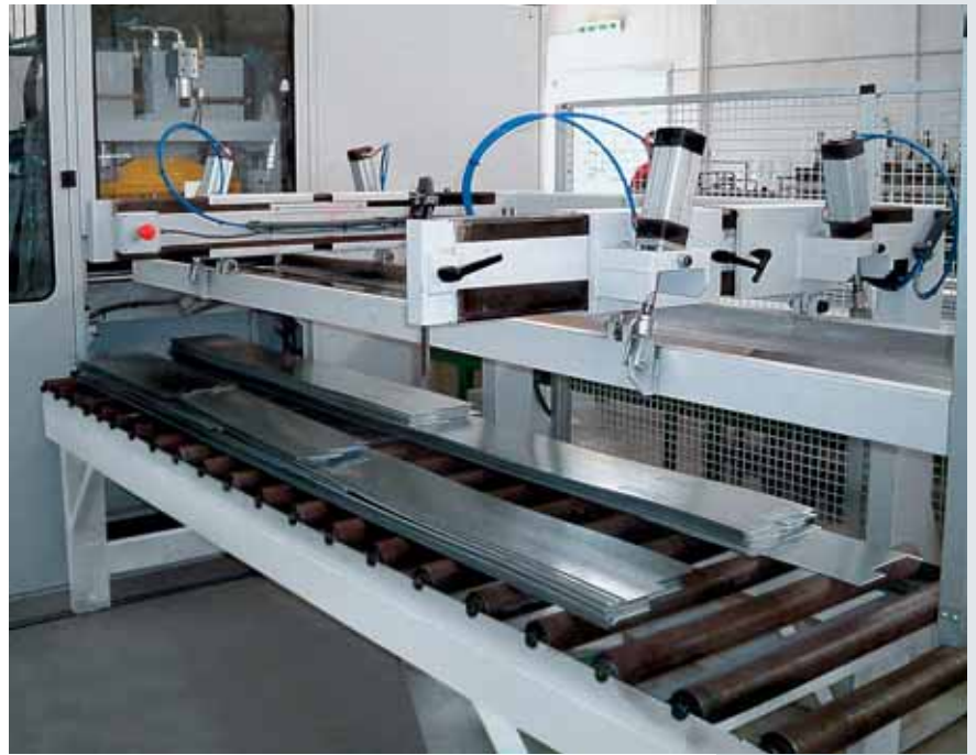
Picture 24 Stacking bench system
